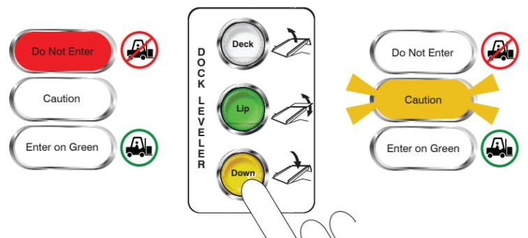
Touch the 'Down' button. Screen will read "Hold to Lower Guard." Hold it for three seconds. Screen will read "Guard Lowering." Control panel light will turn from RED to flashing YELLOW when in bypass mode.
