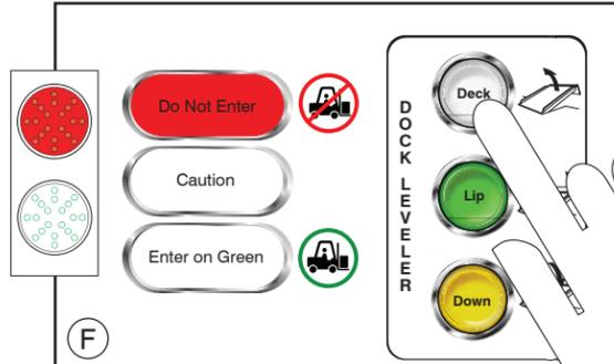
Touch and hold 'Deck' button. Control panel light will turn RED. Deck will raise and lip will retract. When lip has fully retracted, release 'Deck' button. Screen will read "Deck Moving." Deck will lower to home position with lip in lip keepers. Screen will read "Dock Leveler Restored" followed by "Ready to Release" (refers to vehicle restraint).
