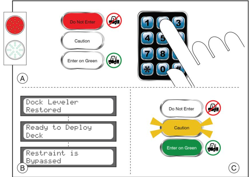
2A) Touch the \* key on the keypad. The screen will read "Enter Code \* \_ \_ \_". Enter the supervisor code.
