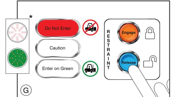
Touch 'Release' button. Screen will read "Restraint Releasing." When vehicle restraint is in the home position, the screen will read "Blue Genius Ready."
