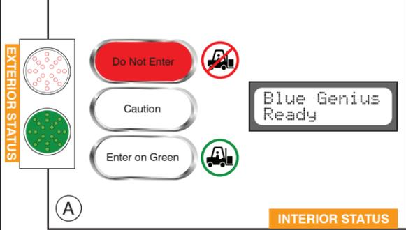
Before truck enters driveway, exterior traffic light will be GREEN and control panel light will be RED. Screen will read "Blue Genius Ready." Truck may now enter driveway. This sequence also indicates that it is safe for truck to depart at the end of loading / unloading.
