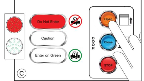
Touch and hold 'Open' button to raise overhead door when door is not in automatic mode. Screen will read "Door is Opening."
