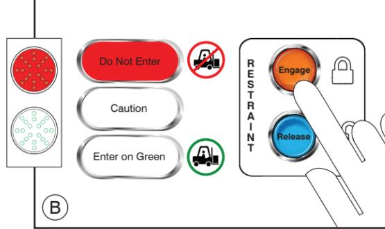
Touch 'Engage' button to activate vehicle restraint. Exterior traffic light will change to RED. Screen will read "Restraint Engaging." Once ICC bar is secured, message will change to "Restraint is Engaged" followed by "Dock Leveler Restored" and "Ready to Raise Deck." If error message appears, see reverse for override instructions.
