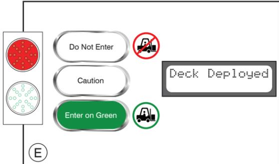
Vehicle restraint and dock leveler deployed correctly. Perform loading and unloading.
