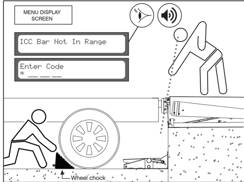
During "Engaging Restraint," the screen may read "ICC Bar Not in Range." This message indicates that a vehicle's ICC bar is absent or cannot be engaged.
