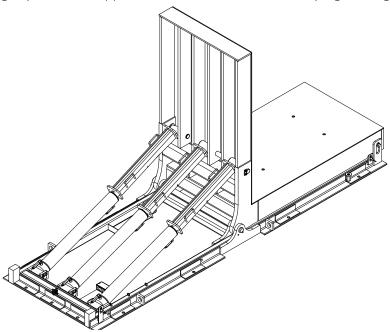
Remove a Service Stand from an exposed section of an extended hydraulic cylinder.
