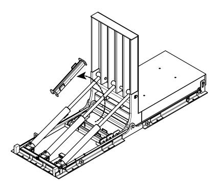
Position the Service Stand onto the exposed section of an extended hydraulic cylinder.
