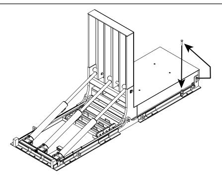
Verify that both Maintenance Pins are solidly stored in the lower frame storage holders before returning to work. Adjust the Maintenance Pins, if required.
