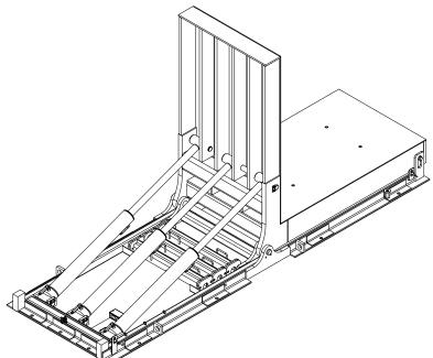
Remove a Maintenance Stand from the holders in the lower frame of the table.
