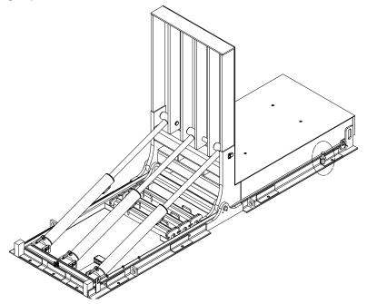
Remove the Maintenance Pin from the holder in the lower frame then attach the Maintenance Pin into the tilt table anchor bracket on each lower frame side.
