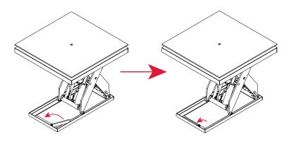
5. Press and hold the **DOWN** button to lower the lift turn table to ground or lowest height position then release the button.
