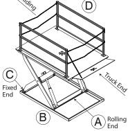
\* Capacities are based on evenly distributed loads. Single axle rolling load capacity is 80% of rated capacity across the ends and 50% of rated capacity across the sides - based on model.
