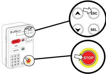
For situations where the dock leveler might need to be stopped immediately, the Blue Genius control station has a 'STOP' button. Touching the 'STOP' button during the operation of the dock or lip will cause the leveler to stop in mid motion.
