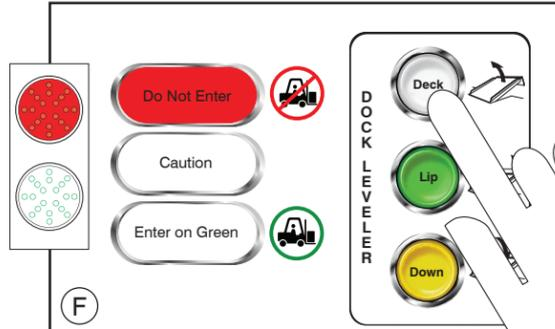
Touch and hold 'Deck' button. Control panel light will turn RED. Deck will raise and lip will retract. When lip has fully retracted, release 'Deck' button. Screen will read "Deck Moving." Deck will lower to stored position with lip in lip keepers. Message will change to "Dock Leveler Restored" followed by "Ready to Release" (refers to vehicle restraint).
