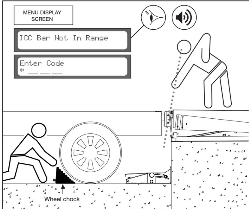
During "Engaging Restraint," the LCD screen may read "ICC Bar Not in Range." This message indicates that a vehicle's ICC bar is absent or cannot be engaged.
