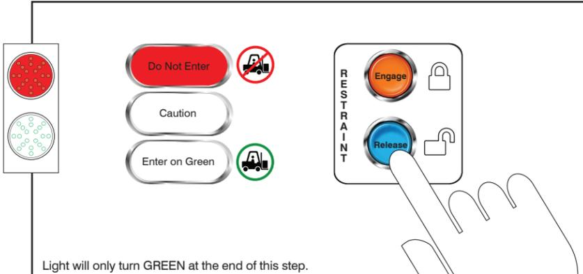
Store the dock leveler. (**NOTE:** Override is still active when dock leveler and vehicle restraint are in the parked position). The control panel light will turn RED
