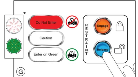
Touch 'Release' button. Screen will read "Restraining Releasing." When restraint is in the home position, message will change to "Blue Genius Ready."
