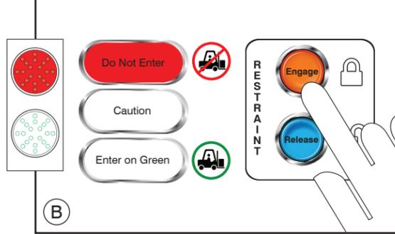
Touch 'Engage' button to activate vehicle restraint. Exterior traffic light will change to RED. Screen will read "Restraining." Once ICC bar is secured, message will change to "Restraining is Engaged" followed by "Dock Leveler Restored" and "Ready to Raise Deck." If error message appears, see reverse for override instructions.
