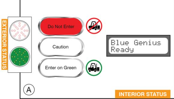
Before truck enters driveway, exterior traffic light will be GREEN and control panel light will be RED. Screen will read "Blue Genius Ready." Truck may now enter driveway. This sequence also indicates that it is safe for truck to leave at the end of loading / unloading.
