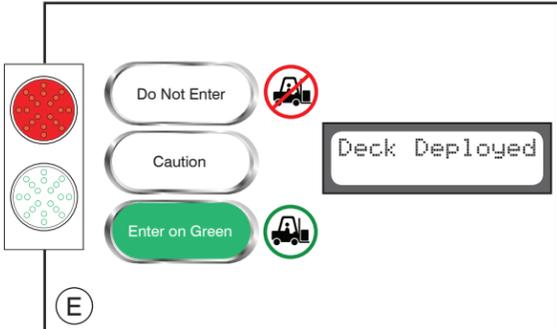
Restraint and leveler deployed correctly. Perform loading and unloading.
