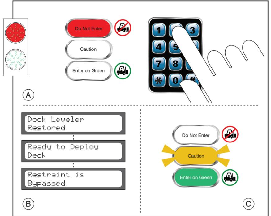
2A) Touch the \* key on the keypad. The LCD screen will read 'Enter Code \* \_ \_ \_'. Enter the supervisor code (default factory set code is '247').
