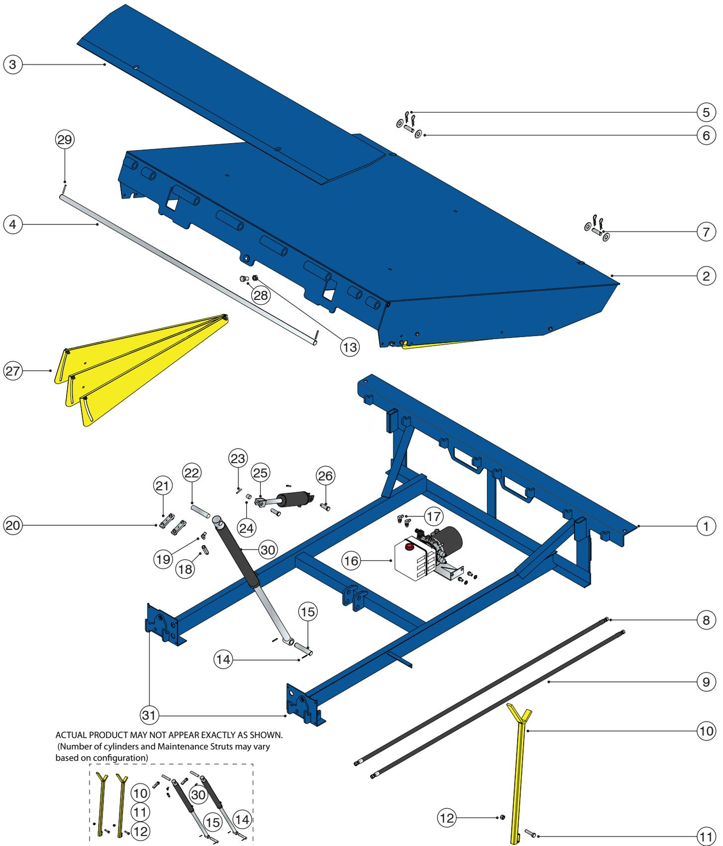
**10.3 MECHANICAL ASSEMBLY - HYDRAULIC DOCK LEVELER**
