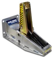
Blue Giant hydraulic vehicle restraints hold trucks securely at the loading dock, improving safety levels during cargo handling operations. Our models are low-profile, have a wide restraining range, and can accommodate a wide variety of ICC bars, including those that are bent or damaged. Comes with the Blue Genius™ Gold Series II Vehicle Restraint Control Panel and traffic lights package.
