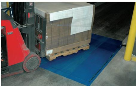
Over 75% of North American trucks are now equipped with air-ride suspension. To ensure compatibility with a broader variety of truck types, Blue Giant offers assured motion float, a 4" (102mm) maintained deck tilt, as an optional alternative to the standard fixed rear hinge. The floating action enables full-width contact between the lip and truck bed, preventing damage to forklift tires and cargo as well as lessening the jarring motion that
